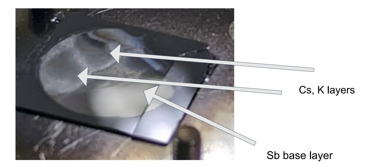
Takeaways: slower deposition from dispensers (to allow gas to diffuse in chamber), lateral position adjustments needed during deposition
