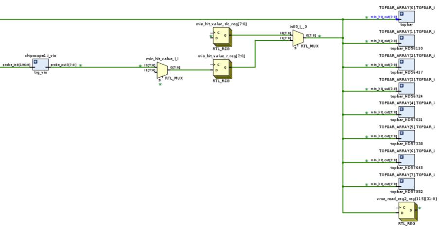
same result (before / after) if an additional register (instead of a multiplexer) is used in a synchronous process
