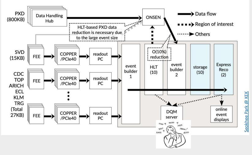
Output of **HLT** (low-level information, timing, triggering etc.) and **Express reco** (w/ PXD and further reconstruction-related) are monitored for DQM.
