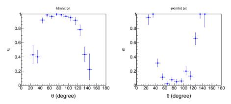
The efficiency for eklmhit, klmhit bits with  $\theta$  distribution.
