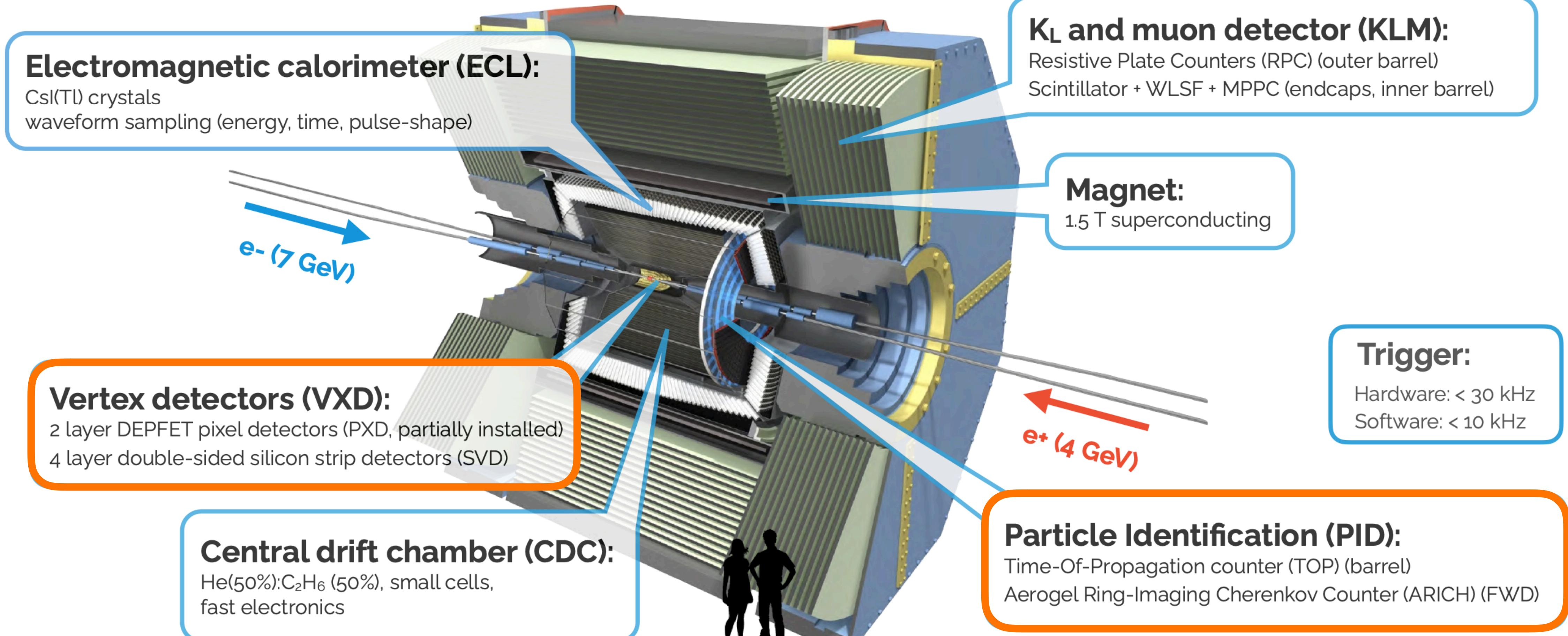
DEPFET: depleted p-channel field-effect transistor
