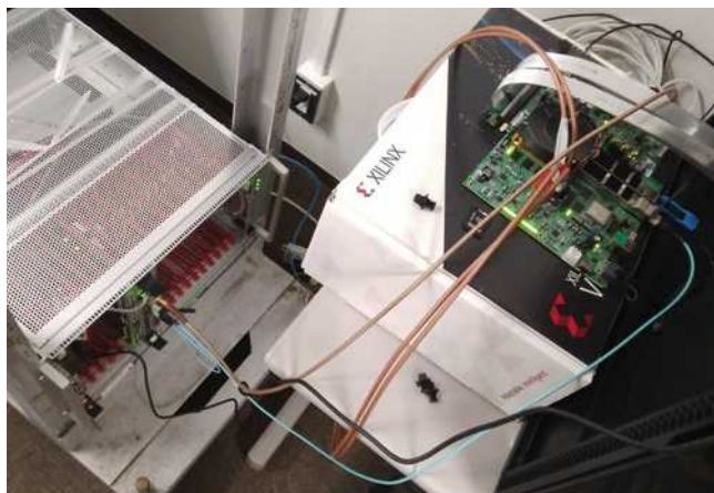
VPK120 connection to Belle II UT4
