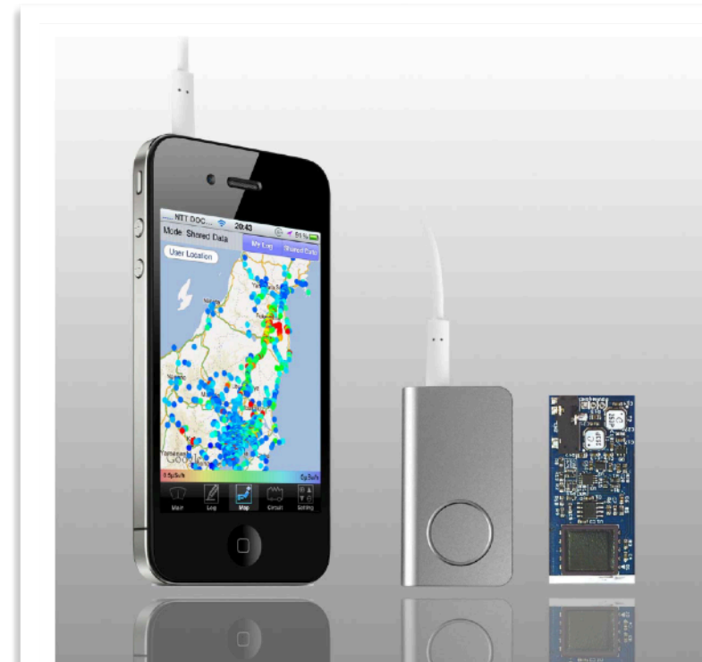
Fig. 1. Pocket Geiger (Type 4) and its PCB.
