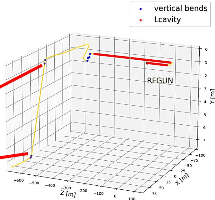
These spin tracking using BMAD show if the electron starts with vertical spin  $(0,1,0)$  at the source, after all the vertical beam motion, it will end up with a vertical spin at the injection point, as desired.
