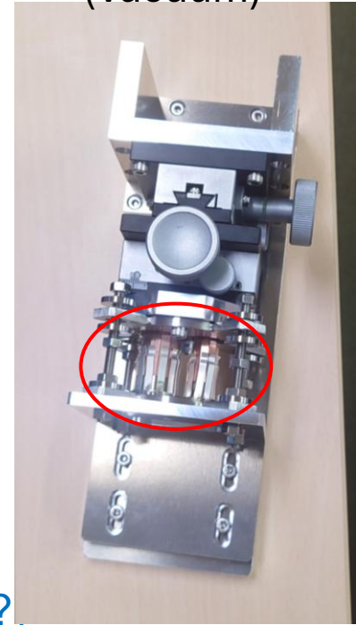
Bellows RF finger test (Vacuum)
