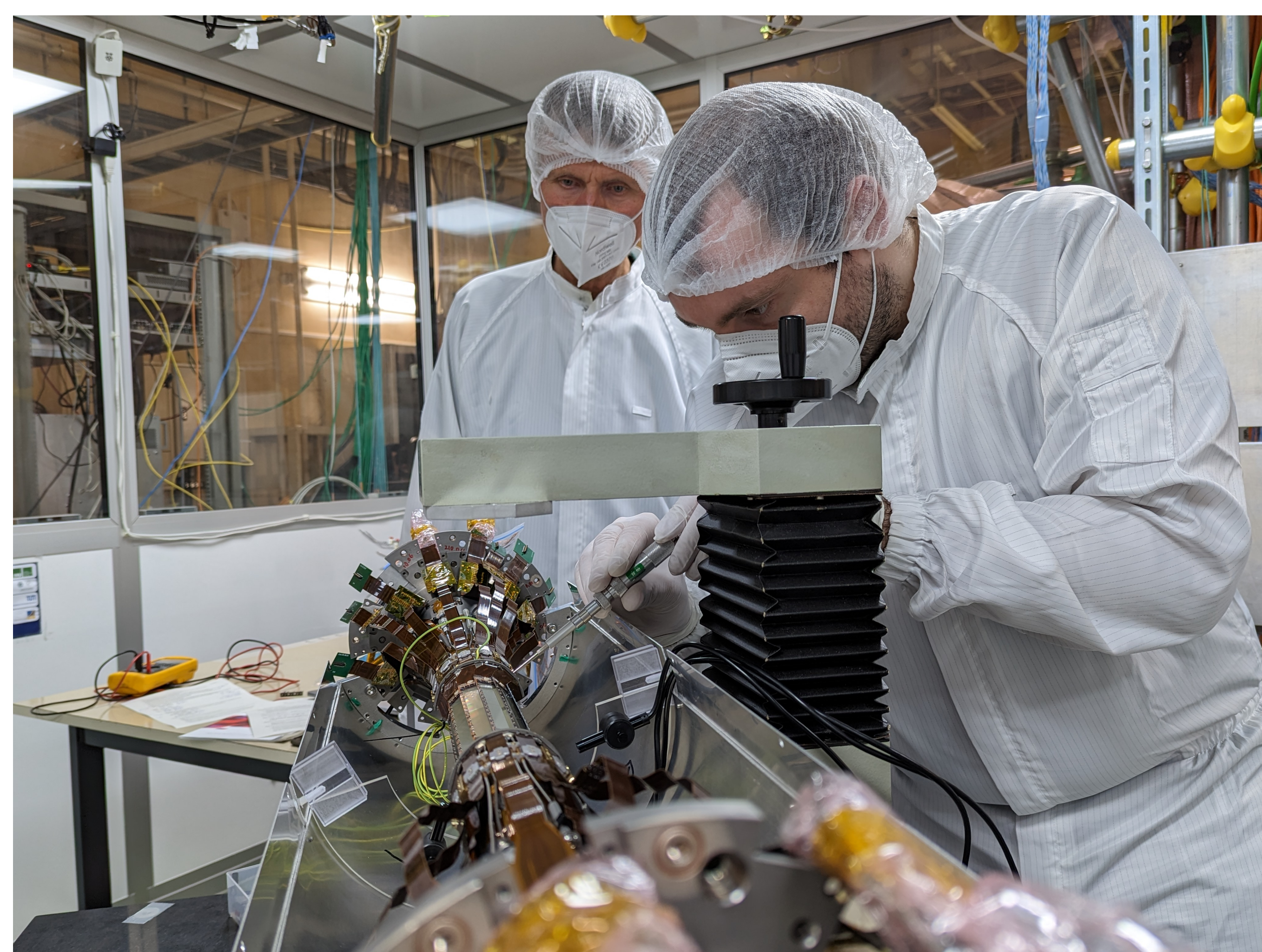
Installation of PXD2 onto the beam-pipe
