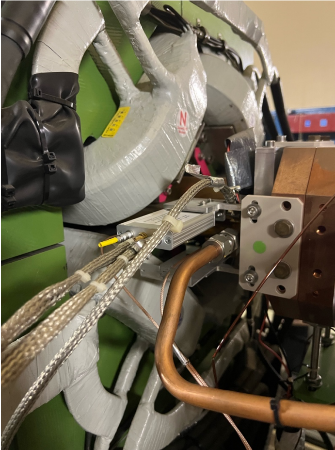
Figure 6: (Left) Top/Bottom config with diamond on the top and LGAD on the bottom. (Right) Diamond sensor a few metres downstream.
