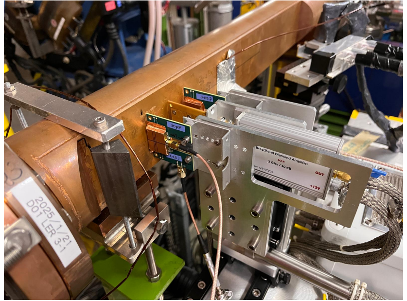
Figure 5b New LGAD installation on LER. 15 pixel LGAD (left) installed on the IR
