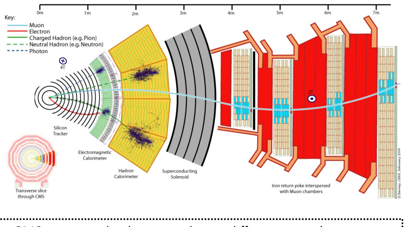
• CMS organised in layers to detect different particles Particle Flow algorithm connects info from sub detectors → precise momentum measurements and particle identification • But... standard algorithms not designed for LL signatures!
