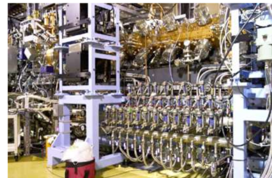
RFQ (Radio Frequency Quadrupole Linac) Up to 50 MeV
