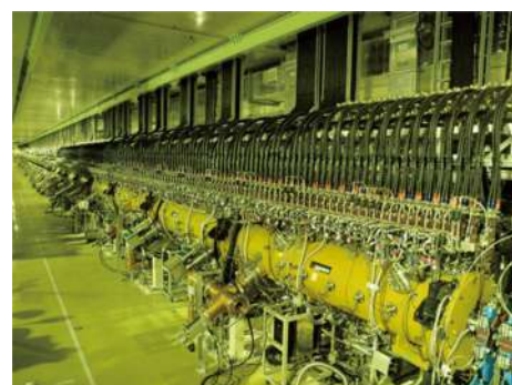
Drift Tube Linac (DTL) Up to 3 MeV
