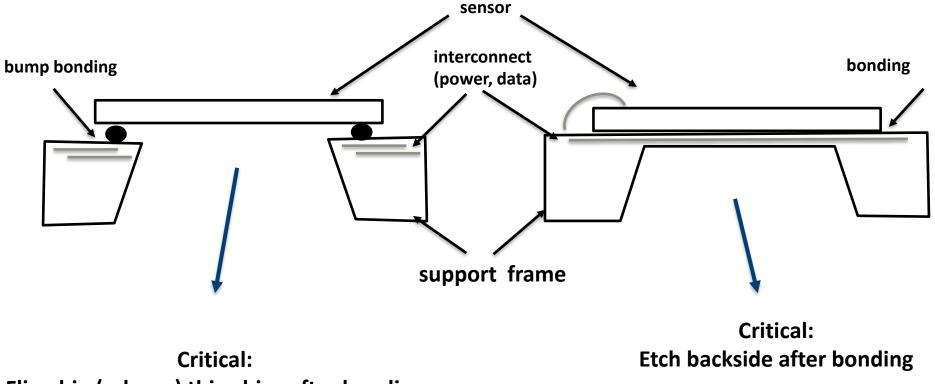
Flip-chip (release) thin chips after bonding
