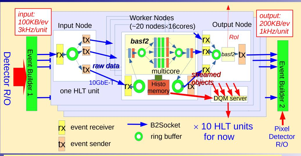
Unit structure (~10 units, 320 CPU cores/unit)
