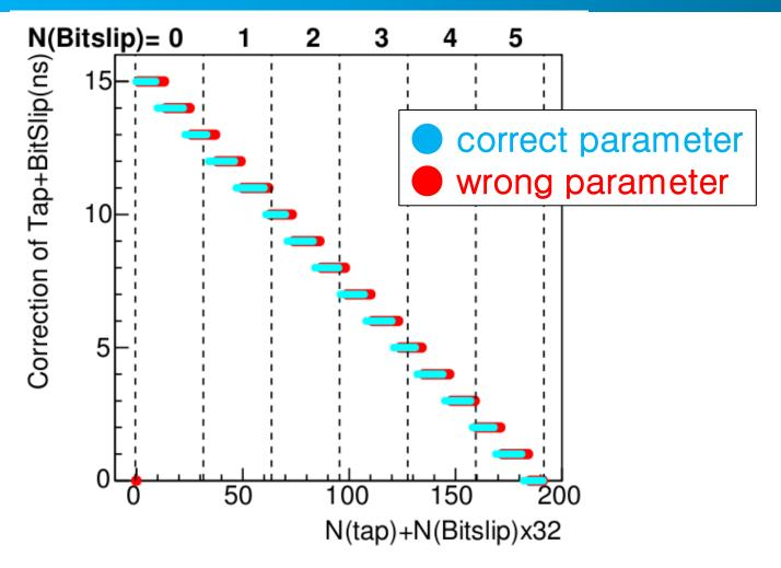
With wrong parameters, 1 or 15 ns TC timing shift happened whenever FPGA was rebooted...
