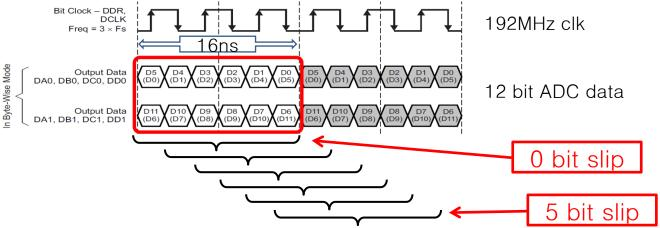
•tap: shift ADC data with 0-31 tap(=0.0-2.3ns) with 75ps interval in order to adjust position of middle of data to clock edge(192MHz).
