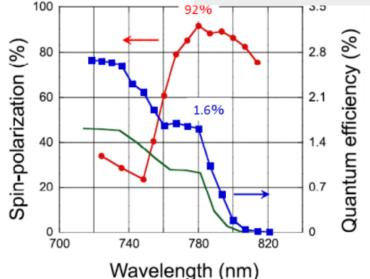
GaAs cathodes can produce beams with >90% polarization and ~1.6% QE, but due to a wide band gap accelerating electrons is difficult
