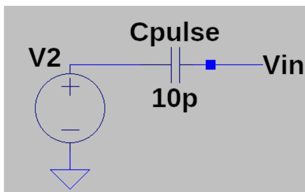
Figure 2.4: Test-charge injection circuit
