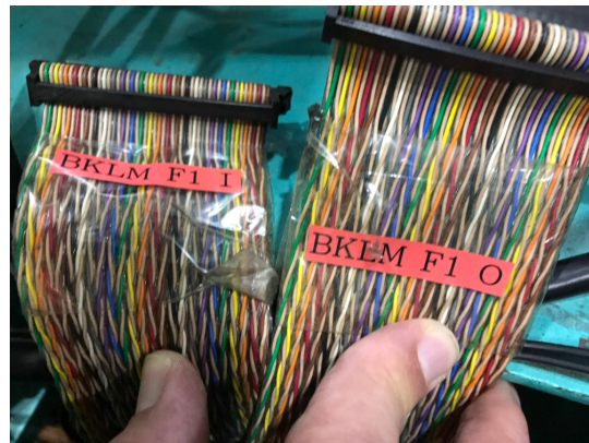
Ribbon cables from bubbler sensor circuit to VME r/o board
