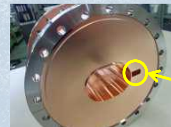
Beam channel for injection
