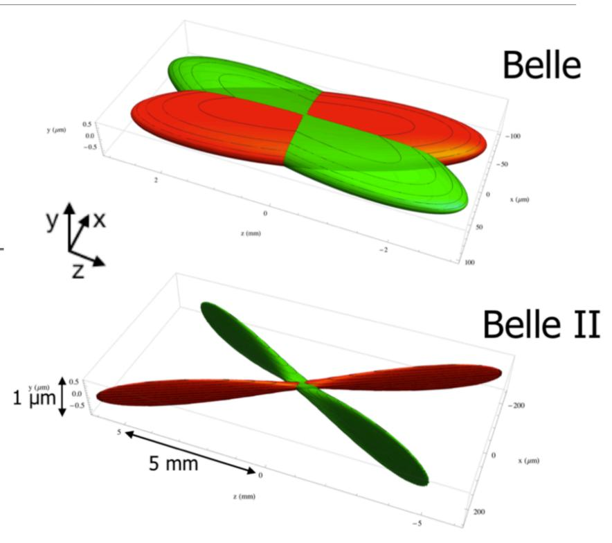
Dimensions of luminous region at Belle II are  $10/0.2/250 \,\mu m (x/y/z)$ compared to  $100/1/6'000 \ \mu m$  at Belle. Ultimately, y size expected to be decreased to ~60 nm
