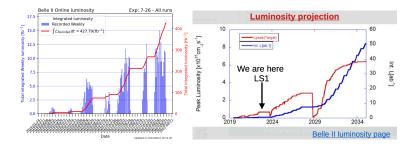
• Shutdown (LS1) from summer 2022 for 15 months: improvement of machine and detector (beam pipe, pixel vertex detector, Time-Of-Propagation PMT)
