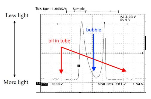
As the edges of the bubble pass through the photogates, they refract the light, causing a decrease in intensity.
