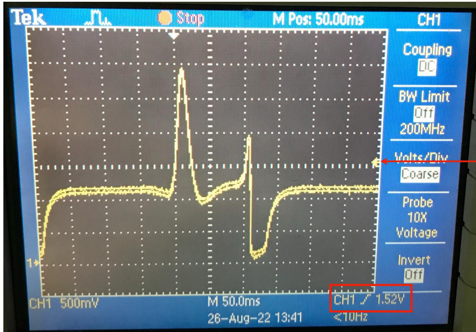
Trigger threshold (1.52V) on rising edge
