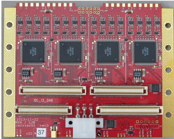
Carrier board – 4 ASIC per carrier
