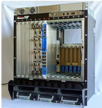
Advanced Telecommunication Computing Architectures (ATCA) Shelf
