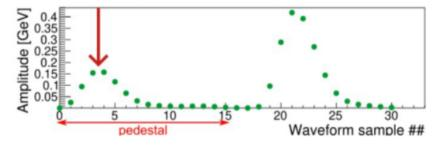
This can be fixed in several ways, best energy resolution is achieved if we save waveform data with bad pedestal for offline re-processing at the ECL unpacking stage.
