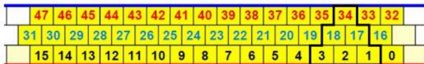
Figure 10: Part of CDC outer SL inside wire cell configuration [6].
