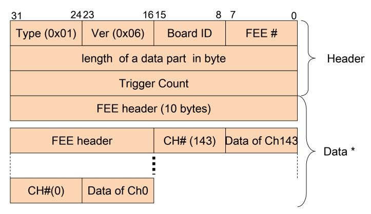
\* If a ch has no hit data (Zero), its data is not transmitted.
