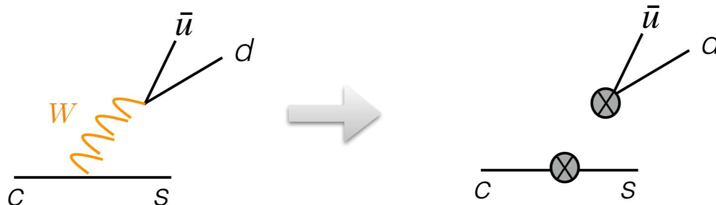
$$A = -\frac{G_F}{\sqrt{2}} V_{cs}^* V_{ud} \frac{M_W^2}{k^2 - M_W^2} (\bar{s}c)_{V-A} (\bar{u}d)_{V-A} \quad (\bar{f}f)_{V-A} \equiv \bar{f} \gamma_\mu (1 - \gamma_5) f$$
