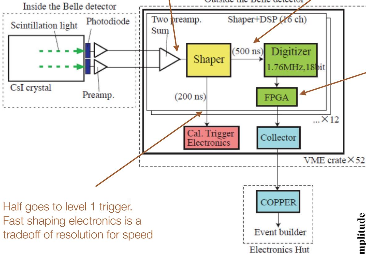
Waveform (i.e. voltage vs time) is fit in FPGA to extract amplitude and time of signal
