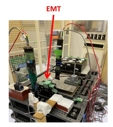
First we need to get the EMT signal from the EMT to an oscilloscope on a computer
